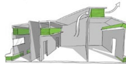
The simplest method of enhancing the acoustics of a vented facade is to place the NVA behind an open-able vent/window. In this instance, the vent/window is used to control the air flow into the building, maintaining the thermal performance of the facade as well as keeping the weather out.
