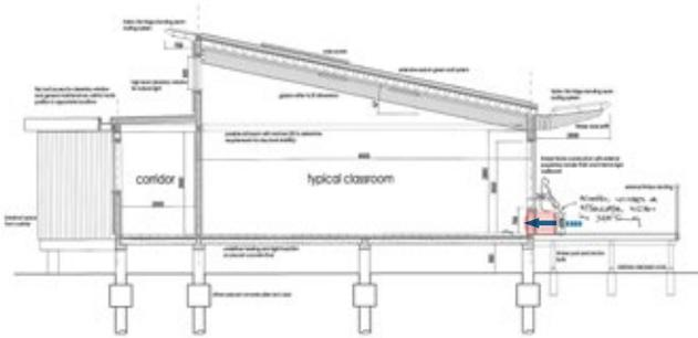
One of the unique elements of this project was a considerable slope across the site. Working with B3 and Craddy Pitchers Davidson, the solution was to pile the site and use suspended slabs to form the classrooms. To provide an external play/learning area to each of the classrooms, a suspended timber deck was employed.
